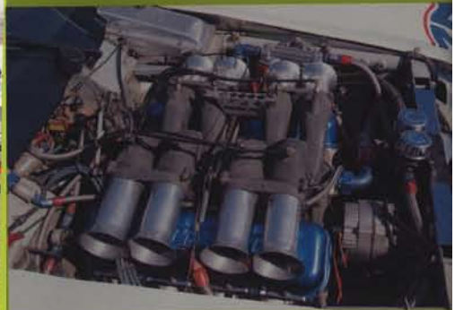
Note the exotic-for-its-time Kinsler mechanically fuel-injected cross-ram manifold on an all-aluminum 427 in the Greenwood car. According to Greenwood, these engines made 700 hp back in 1975.
